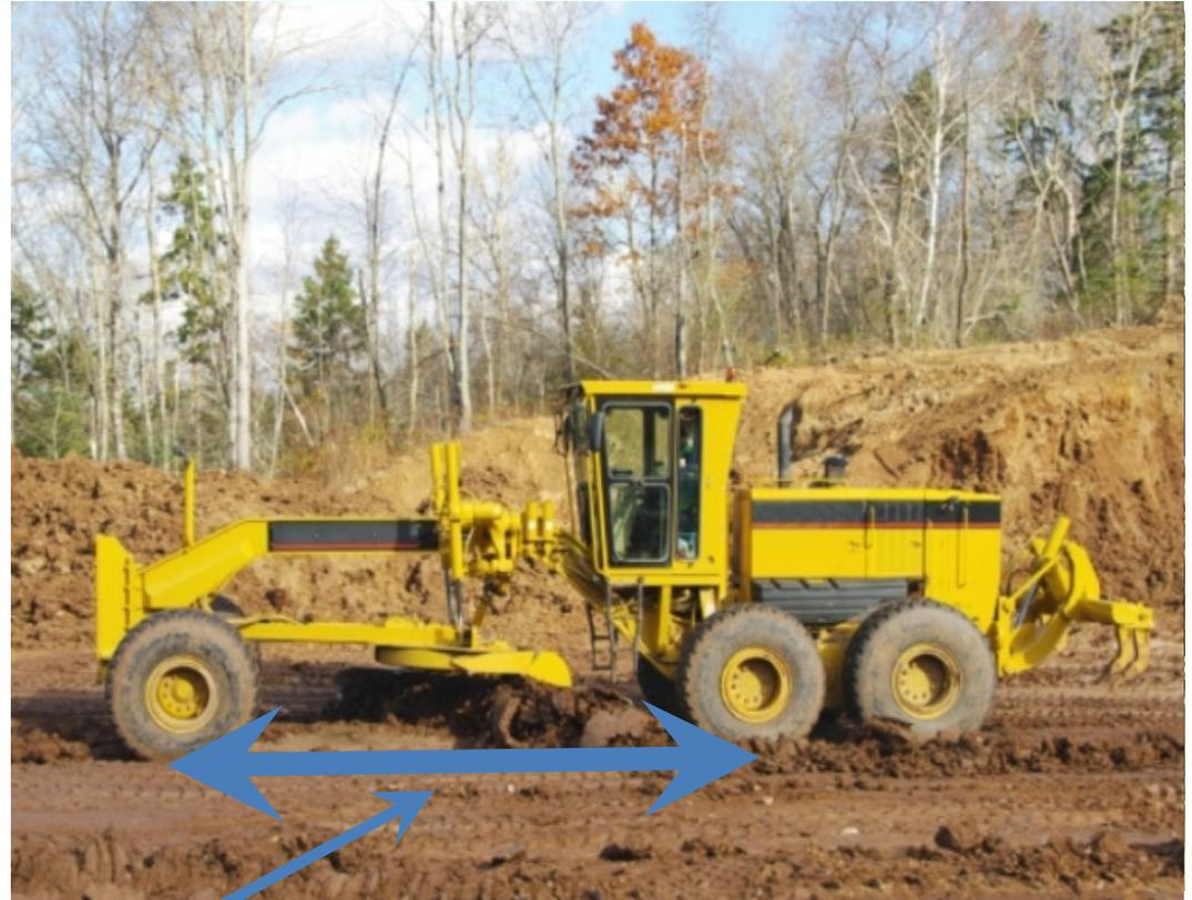
Long span relative to the size of the bumps to be removed
